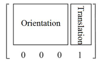
Simply, the Orientation part is represented by a special orthogonal matrix, and the translation part is represented by a vector.
