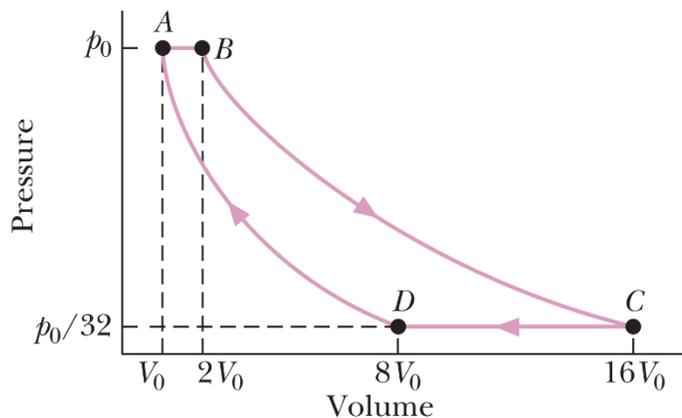
4 | In the figure below, 3 moles of an ideal diatomic gas undergoes different processes in a thermal-engine. Starting from point  $a$ , it goes through an isobaric process to point  $b$ , and having an isothermal process to point  $c$ , it reaches to point  $d$  via an isovolumetric process, and finally completes the cycle experiencing an adiabatic process.
