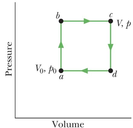
3 | An ideal gas ( $1.0 \text{ mol}$ ) is the working substance in an engine that operates on the cycle shown in the figure. Processes  $BC$  and  $DA$  are reversible and adiabatic.
