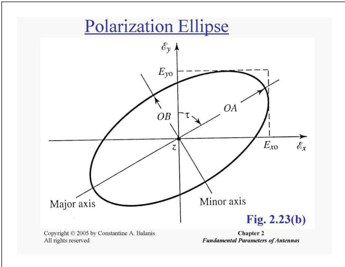
The figure of the electric field is traced in a clockwise (CW) or counter-clockwise (CCW) sense. Clockwise rotation of the electric field vector is designated as *right-hand polarization* and counter-clockwise as left hand polarization.
