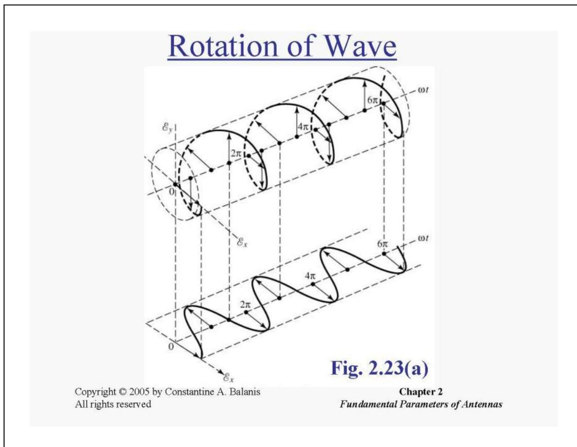
We have, in general **elliptic polarization**. **Linear** and **circular** polarizations are special cases.
