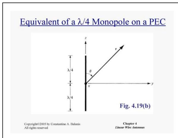
$P_{rad}$  only above ground, half of the power of half-wave dipole.
