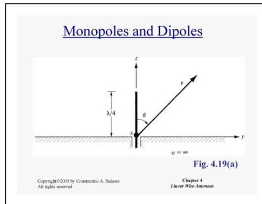
Monopole of  $\ell = \frac{\lambda}{4}$  above the ground is equivalent to the half-wave dipole for above the ground.
