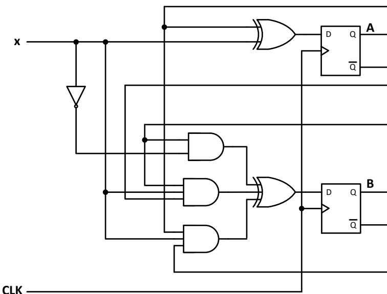
$$\underbrace{A(t+1)}_{\text{next state}} = D_A = \underbrace{A(t)}_{\text{present state}} \oplus x$$
