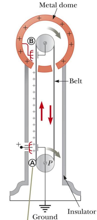
The charge is deposited on the belt at point A and transferred to the hollow conductor at point B.
