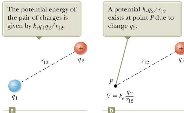
The potential energy of the system is  $U = k_e \frac{q_1 q_2}{r_{12}}$ .
